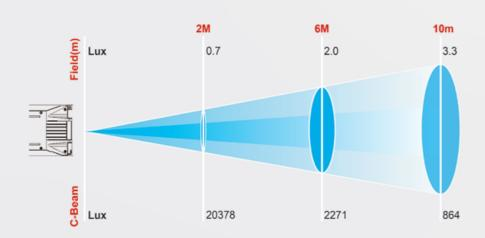
The light not only be sharp, framing shutters and gobo or plastic slides projection, but also have intense accent light output and silence working environment. Beam angle can be selected 19°/26°/36°/50°, you can exchange lens of our this light with ETC's
