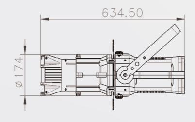
The light not only be sharp, framing shutters and gobo or plastic slides projection, but also have intense accent light output and silence working environment. Beam angle can be selected 19°/26°/36°/50°, you can exchange lens of our this light with ETC's
