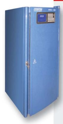
SRD-48 is a 48 channel network/optical fiber dimmer rack suitable for TV studios, theater halls and conference centers with a capacity of 24 dimmer modules. Each dimmer module supports two dimmers of maximum 6KW output per channel. SRD-48 accommodates sine wave modules in addition to phase control and relay modules.
